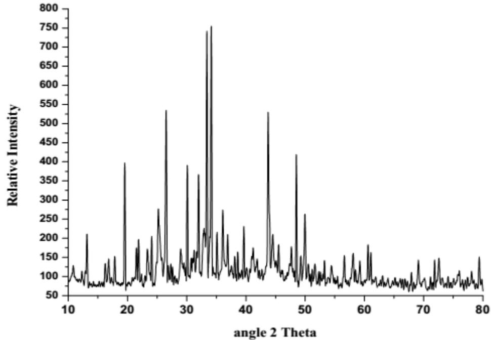
*Fig 1: XRD structure of  $\text{MgCuAl}_{10}\text{O}_{17}$  Phosphor*
